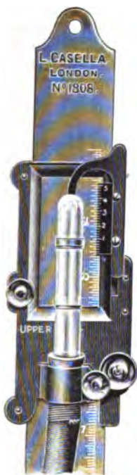
THE UPPER CARRIAGE AND VERNIER, WITH BAROMETER ATTACHED.
